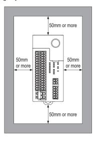
Do not install the unit above devices which generate heat such as heaters, transformers or large scale resistors.
