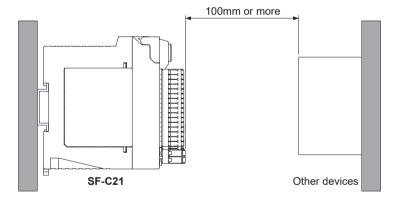
To connect the software tool and cables, keep a space of 170mm or more away from the installation surface of this device.
