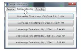
Clicking the bar of a log to be confirmed opens a different screen, allowing you to confirm the logic.
