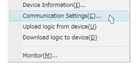
Baud rate, parity bit, stop bit, and addresses can be set.
